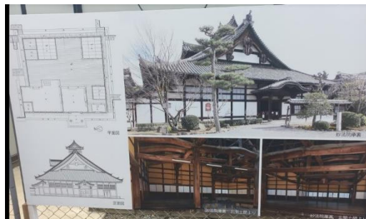
Plan view and wooden structure of the Myoho-in Temple Kuri in Kyoto.
